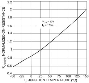
Fig. 4 On-Resistance Variation with Temperature
